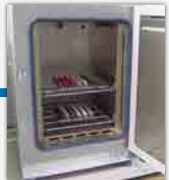
*Samples prepared for ageing in oven at different temperature.*
