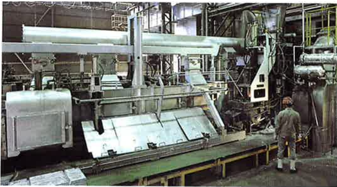
The continuous galvanising system processing conduits shell
