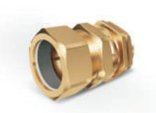
Brass gland suitable for steel tape armoured, plastic or rubber sheathed cables. Terminates and secure cable armouring and outer seal grips sheath of cable thus ensuring mechanical strength and earth continuity.
