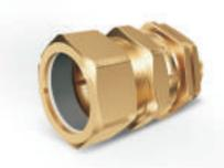
Brass indoor and outdoor gland most popularly used with single wire armoured, plastic or rubber sheathed cable. Terminates and secured cable armouring and outer seal grips sheath of cable thus ensuring mechanical strength and earth continuity.
